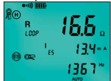
The 2 Clamp method displays clamp connection resistance, test current and frequency.
