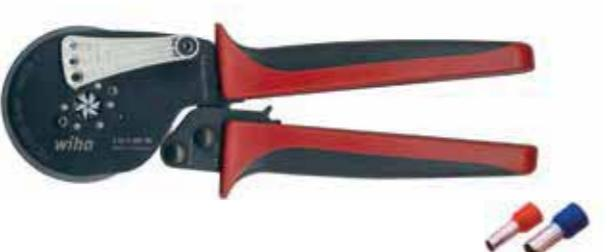
**Lowers your costs:** An integrated lever enables users to interrupt the crimping process at any time to protect the pliers. **Increases your safety:** Safe work through feed aid prevents crimping the plastic cover of wire-end sleeves. **Facilitates your handling:** Thanks to hexagonal crimping, small wire-end sleeves no longer get caught. **Increases your efficiency:** Automatic adjustment of wire-end sleeve size with suitable crimping force for a large coverage area of 0.08-16mm<sup>2</sup>.
