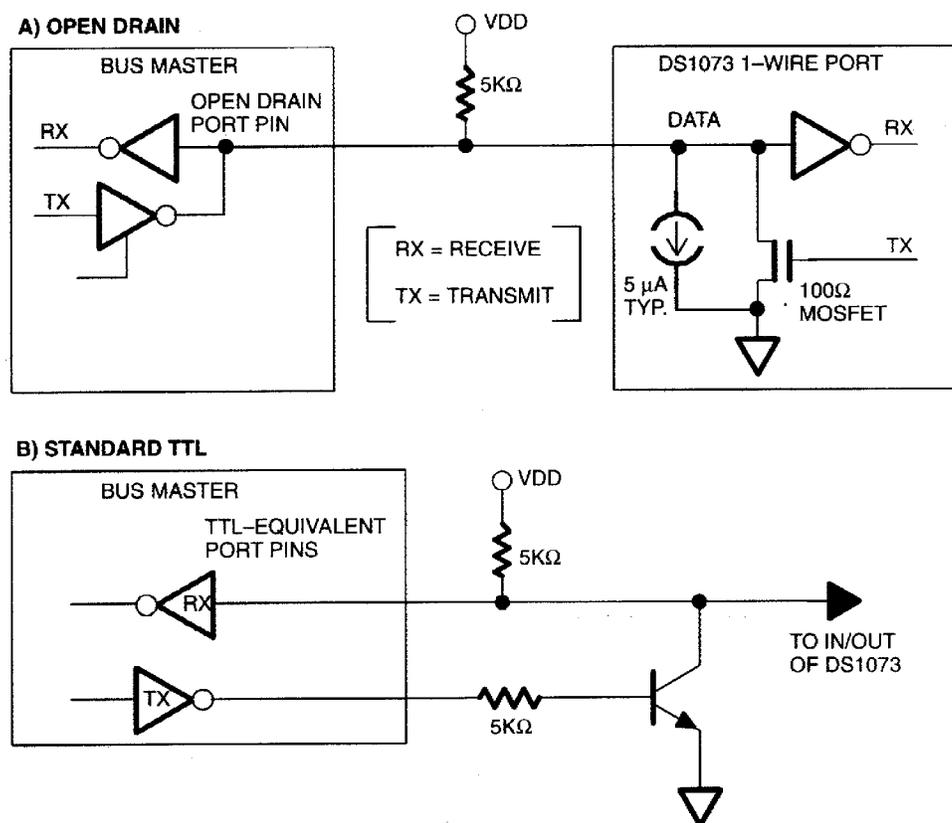
Programming mode is entered by simply powering up the DS1073 with a pullup of approximately 5kΩ. This will pull the I/O pin above  $V_{IH}$  on power-up and initiate the programming mode, causing the DS1073 to internally release the I/O pin (after  $t_{POR}$ ), and allow the pullup resistor to pull the pin to the supply rail and await the Master Tx Reset pulse (see diagram).
