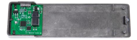
3. Insert the Apple SSD into the black SATA connector on the circuit board, as shown below. The connector is notched so that only one orientation can be used.
