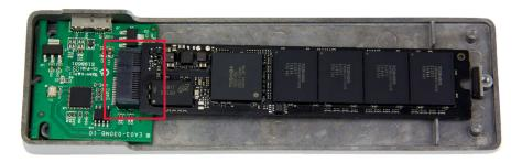
4. Reseat the bottom cover, then use a Torx T5 driver to install the two screws mentioned in **Step 1**. The longer screw goes on the left, the shorter screw goes on the right. Avoid overtightening the screws, as they may strip.
