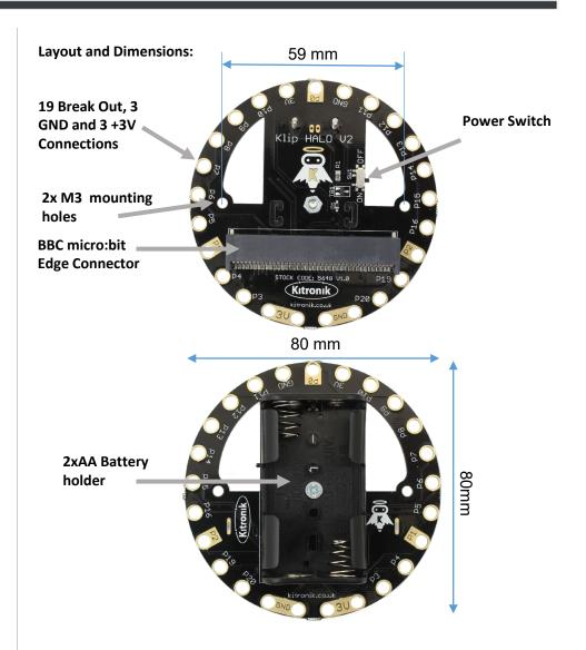
The Klip Halo board is 28.3mm thick (including BBC micro:bit connector and Battery holder)
