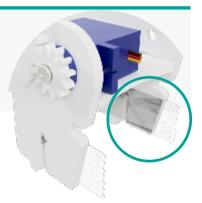
**NOTE:** If you do not have any tape available - you will need to disassemble your :MOVE mini and follow the instructions from the original :MOVE mini manual. Simply replace the two inner side panels with this module you have just built.
