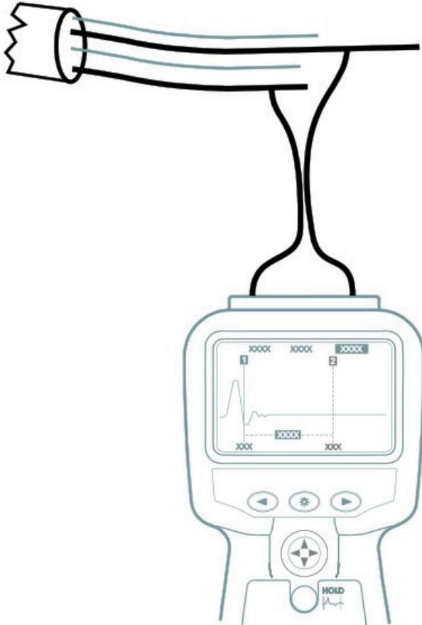
Connect the test lead to the cable under test. Connection may be made to a live power system with a voltage to earth (ground) less than 150 V with an installation (over voltage) category of I V or lower.
