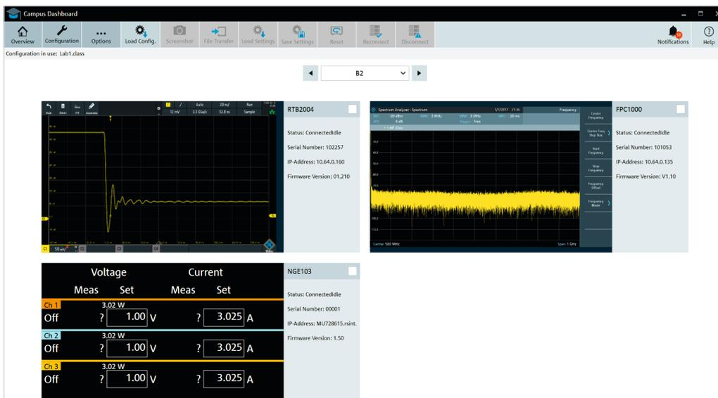
View all instruments on one bench on your computer screen using the R&S®CDS campus dashboard software; the software also supports remote control of each instrument
