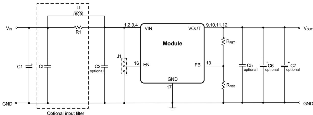
The 171011801 integrates both the input and output capacitors. Therefore, additional external input/output capacitors are normally not required.
