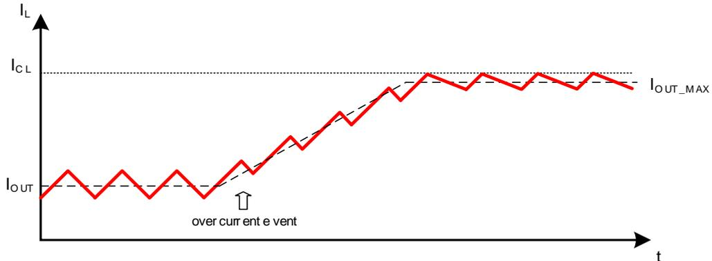
During overcurrent condition, the duty cycle is no longer determined by the control loop, it is instead limited by the current limit threshold. Therefore, the output voltage is out of regulation and drops (see figure below).
