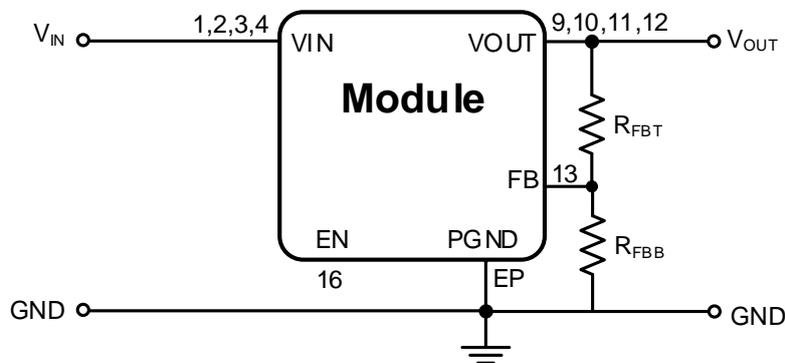
The only external components necessary to operate the 171011801 that must be placed on the PCB are the resistors of the output voltage divider, as shown in the picture above.
