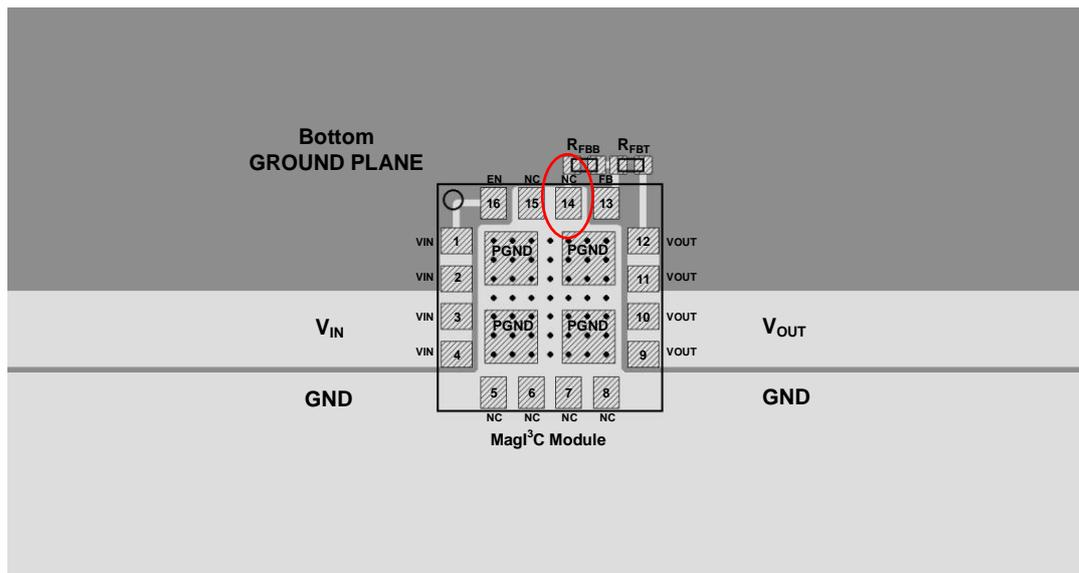
The ground connection of the lower resistor of the output voltage divider ( $R_{FBB}$ ) should be routed to the PGND pins of the device. If not properly handled, poor grounding can result in degraded load regulation or erratic output voltage ripple behavior.
