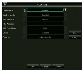
Set the parameters, in the preview interface to select the channel needed to be controlled, and then in the [right-click menu]  $\rightarrow$  [PTZ control] icon to control the camera's menu function application. As shown below.
