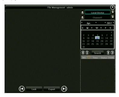
Playback mode will automatically switch to "File Management", after the interface is refreshed, click the button in the lower right corner to retrieve the same day the channel 1 all the capture file, the default channel number sort, followed by the file style.
