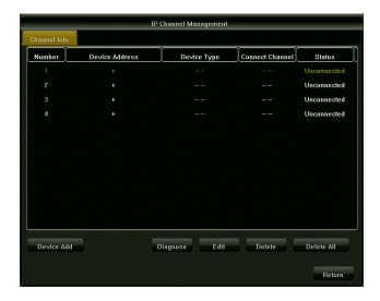
Click on the channel "+" button, HVR will automatically search all IPC in the LAN, search completed, double-click the IP address which is needed to add to the HVR. You can also click on the manual adding, manually enter the IP address and port to add the IP camera.
