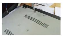
3.Fix the hard disk to the lower shell of the housing with screws.
