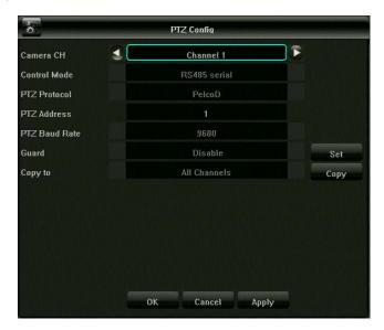
After setting the parameters, select the channel that need to be controlled, in the preview interface, and then in the [right-click menu] → [PTZ control] icon to control the direction of the lens; focal length, focus, aperture zoom in and zoom out; PTZ speed settings. Advanced functions can be set in the lower right drop-down menu. As shown below
