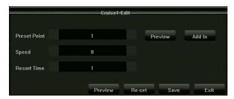
And then select the preset point, cruise speed, retention time, click the "join" button, set the cruise path preset point(you can add multiple preset points).
