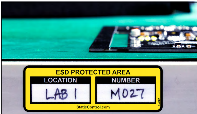
Figure 9. Applying a measurement location label to the edge of a workstation
