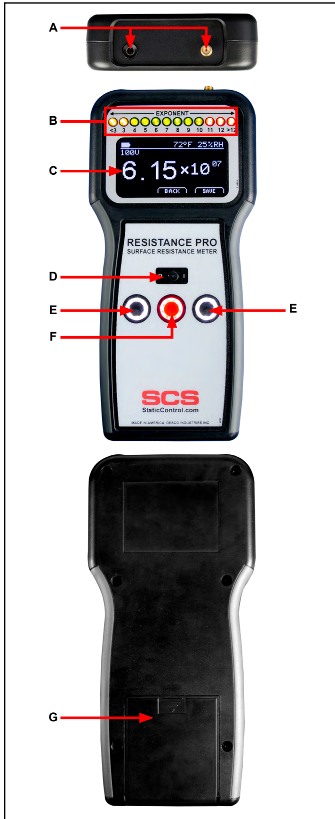
Figure 4. Resistance Pro Meter features and components
