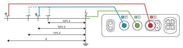
The 3 measurement results must be the same to within a few percent. If this is the case, the measurement is valid. If not, it is because the S rod is in the zone of influence of the earth electrode.
