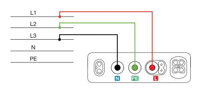
The phase-to-phase voltages are displayed, the values  $U_{12}, U_{23}$  and  $U_{32}$  in cyclic succession, along with the direction of phase rotation,  $L_{3,12}^{L_{1,1}}$  or  $L_{1,12}^{L_{3,1}}$ .
