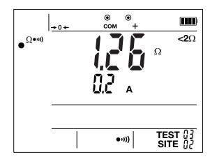
For as long as the measurement varies between some value and OL, the instrument remains on even if not in permanent mode.
