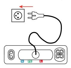
The measurement is displayed. The instrument indicates that it is making the measurement between the L and N terminals. It is therefore possible to make the measurement with two leads.
