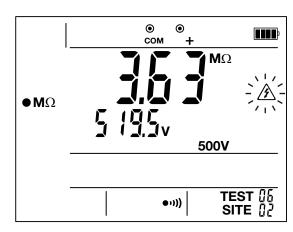
When you release the **TEST** button, the instrument displays **dIS** (discharge) to indicate that it is discharging the object tested. If the object is not capacitive, discharging is very rapid. When the voltage falls below 25V, the **dIS** and  $\triangle$  symbols disappear from the display unit.
