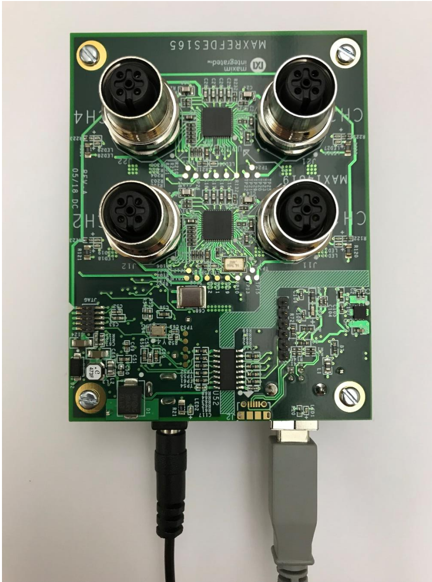
Figure 3. Connect the Power and USB cables to MAXREFDES165# and then connect it to the PC.
