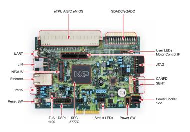
Figure 1: Top elevation of MPC5777C Development Board
