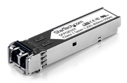
The SFPGESST is a Cisco SFP-GE-S compatible fiber transceiver module that has been designed, programmed and tested to work with Cisco® brand switches and routers. It delivers dependable 1 GbE connectivity over fiber cable, for 1000BASE-SX compliant networks, with a maximum distance of up to 550 m (1804 ft).
