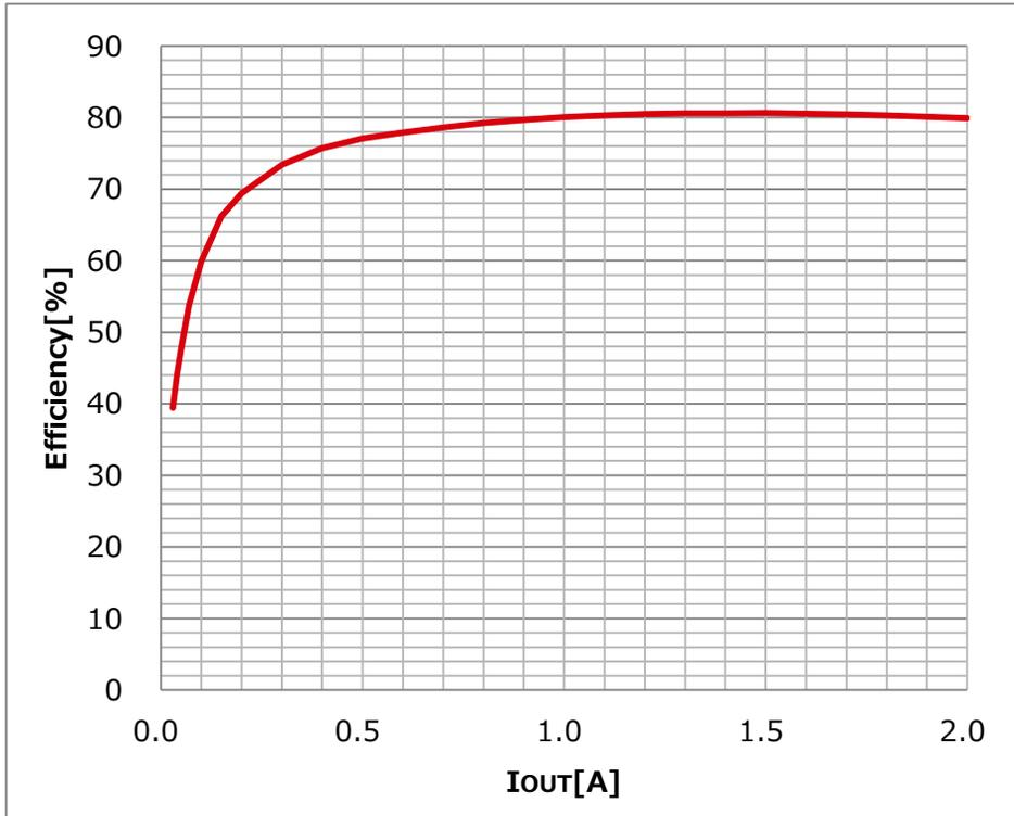
Figure 11. Efficiency vs Load Current
