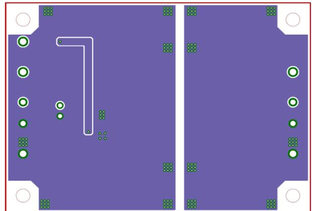
Figure 10. Bottom Side Layer Layout
