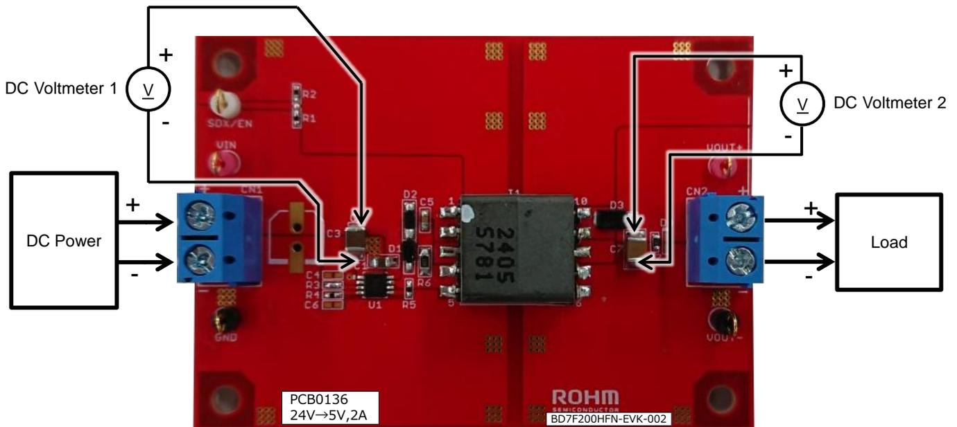
Figure 3. Connection Diagram
