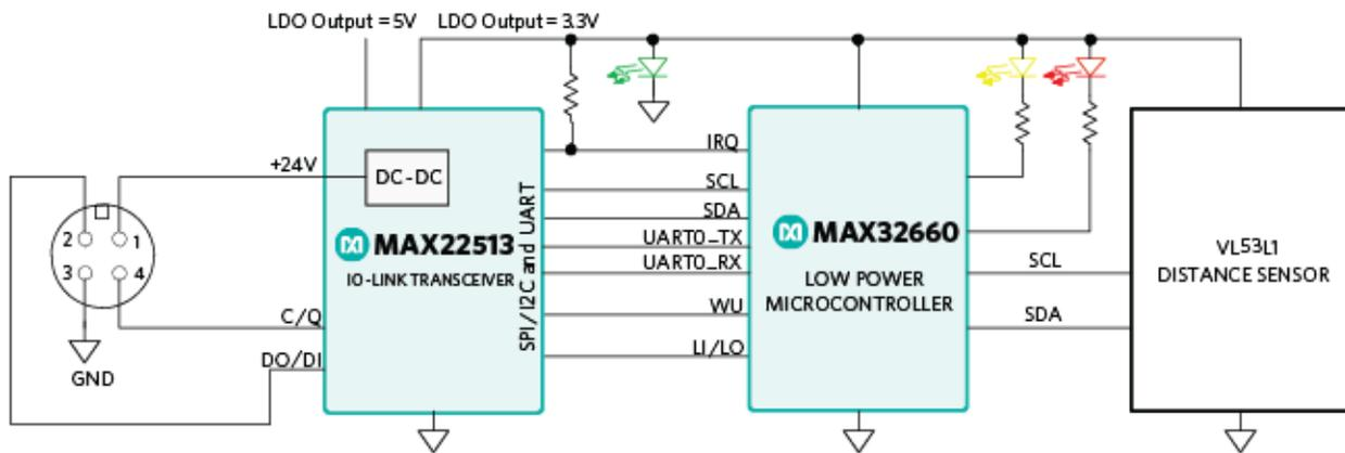
Figure 1. The MAXREFDES171# reference design block diagram.
