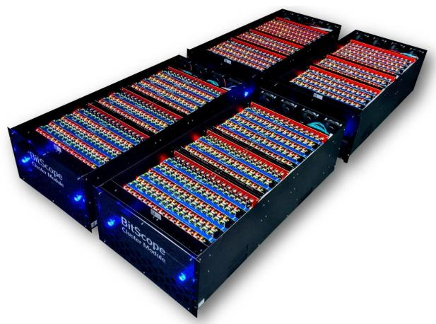
Available in 48, 96 and 144 node sizes, they use the same power and mounting solution as the Large Blade Racks but they also include an integrated network fabric with up to 60Gb/s external bandwidth, built-in power supplies and rack stackable cooling systems.
