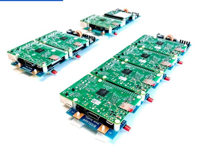
Blade Quattro is one of three BitScope Blade industrial motherboards for Raspberry Pi.
