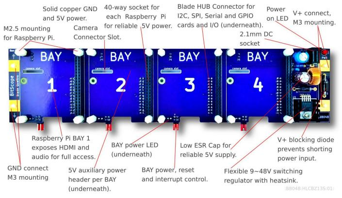
Blade Quattro provides four mounting BAYs for up to four Raspberry Pi.
