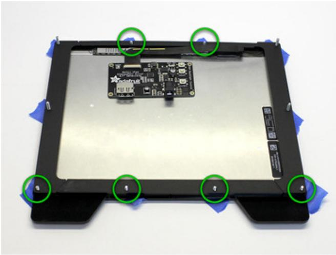
With the edge pieces in place, six nuts can be installed over the shorter (1/2") screws, in the positions marked here. The four longer screws should not receive nuts yet!
