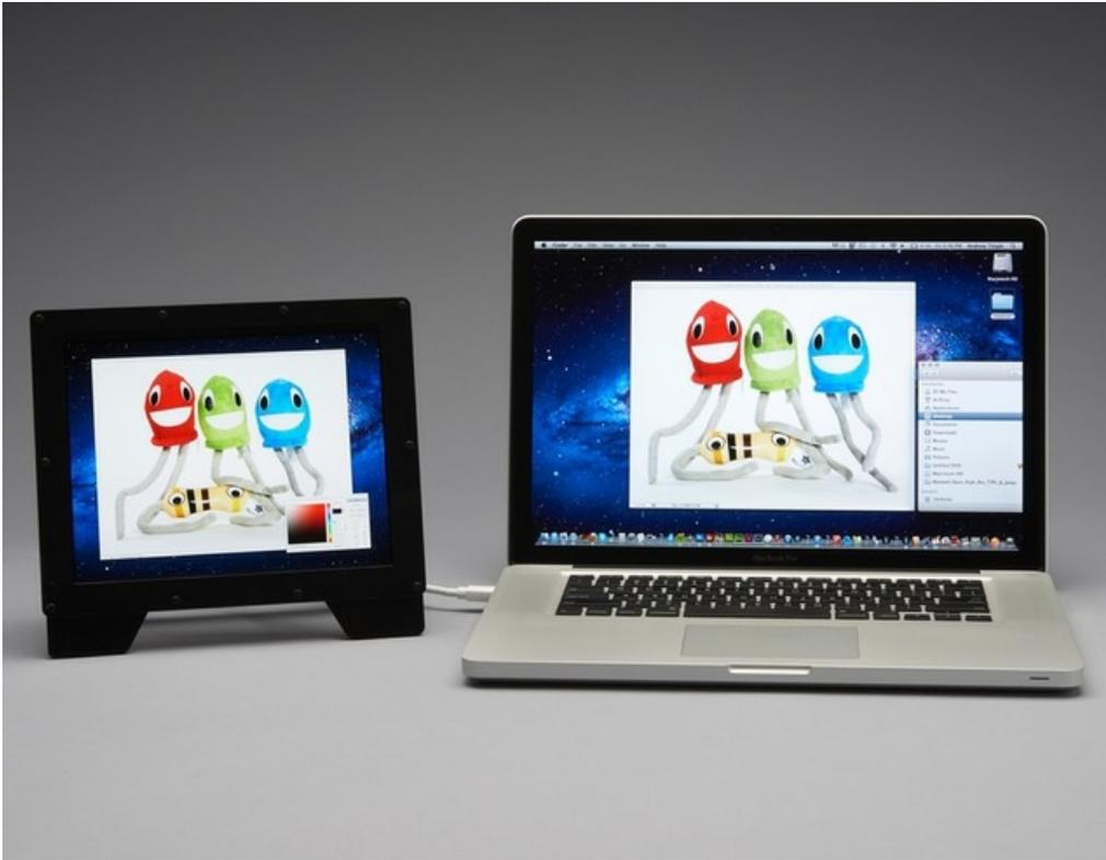
Add a glorious 2048x1536 retina-blasting, ultra-high pixel density, IPS display to any computer with a Thunderbolt/DisplayPort port. This product comes with a new 9.7" diagonal TFT display module (the same one used in the iPad 3 & 4), along with our custom made driver board, a stand-up monitor enclosure kit, 10' DisplayPort cable and 9V power adapter.
