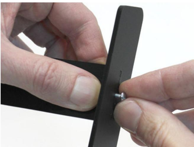
Slots in the leg pieces are "keyed" to fit into the tabs on the cross brace. Position a leg using these tabs and slots, then install a #4-40 1/2" screw through the middle, meeting up with the nut held in the cross brace.
