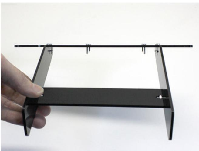
To reiterate a prior point: these screws should sit flush, pointing **back**, not forward. Getting this wrong will break the LCD!
