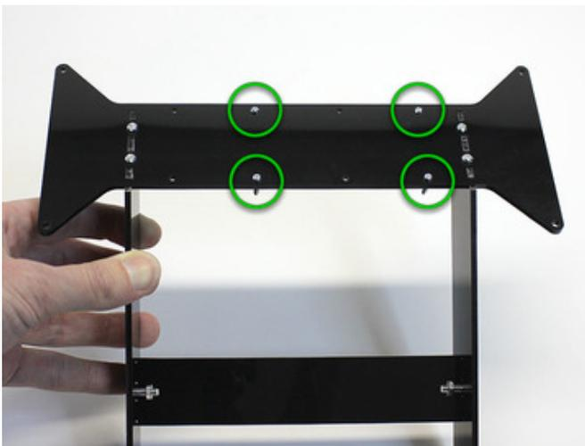
The "bow tie" has eight holes in it, but we'll only be using **four**. Looking at the flat side (the legs should poke out the back, not forward), install the four tiny #2-56 screws in the positions indicated here.
