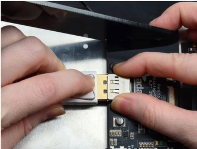
Removing a DisplayPort connector is a little more difficult because the connector is quite strong. You have to press down on the cable latch and wiggle-pull it out. Hold onto the connector with your other hand to make it easier!
