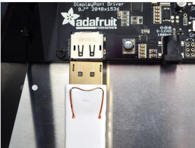
OK plug in your cable so that it snaps in nicely into the DP connector on the Qualia driver. It should snap in all the way
