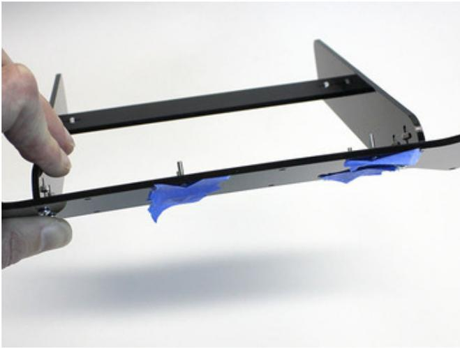
As with the main bezel, a little tape over the heads of these screws helps keep them in place.
