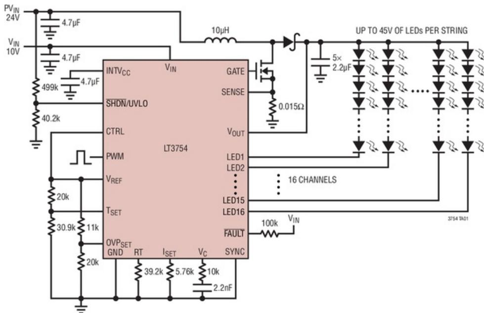
To control the backlight, we use a very tiny microcontroller (the ATtiny85 from AVR) which listens for button presses and then sends a 4KHz PWM signal to the LT3754 to tell it how much to dim the display.
