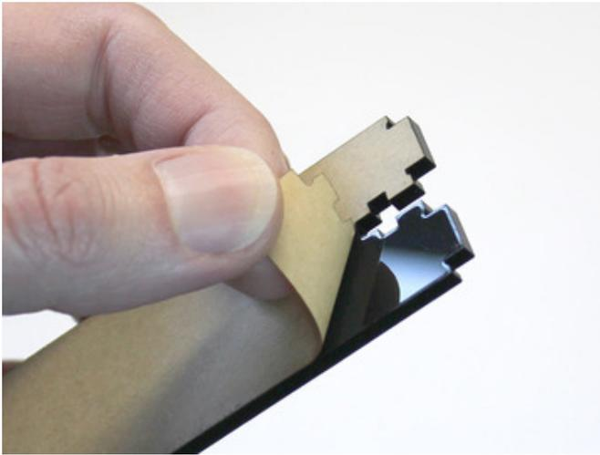
Start by peeling the backing paper off both sides of all the laser-cut parts. It's easiest to start at a corner, catching the edge of the paper with a fingernail.
