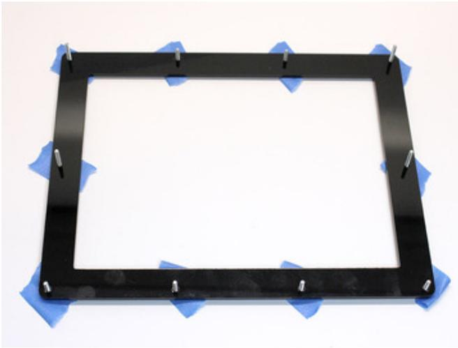
Once all the screws are placed, set the bezel face down on your work surface. Turn it so the “top” (with the longer screws) is at the...well...*top*.
