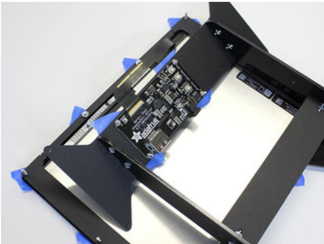
Set the “bow tie” carefully near the top of the screen. Pick up the driver board and...being very mindful of the flex cable, don't tear or pull it out...lower it on to the four small screws on the bow tie. Then add a nut for each.
