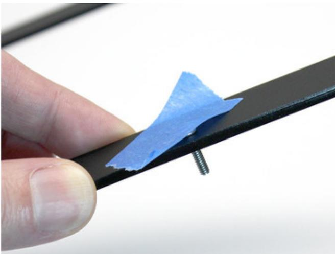
Insert a screw into each hole (1/2" or 5/8", as appropriate to the above diagram). The bezel will need to be flipped over later, so as you place each screw, secure it with a bit of tape, or you can use the nuts temporarily to keep the screws from sliding out (you'll need to remove these nuts later).
