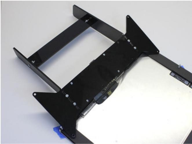
Now flip the bow tie / support over, remove the tape and tighten the four small screws.
