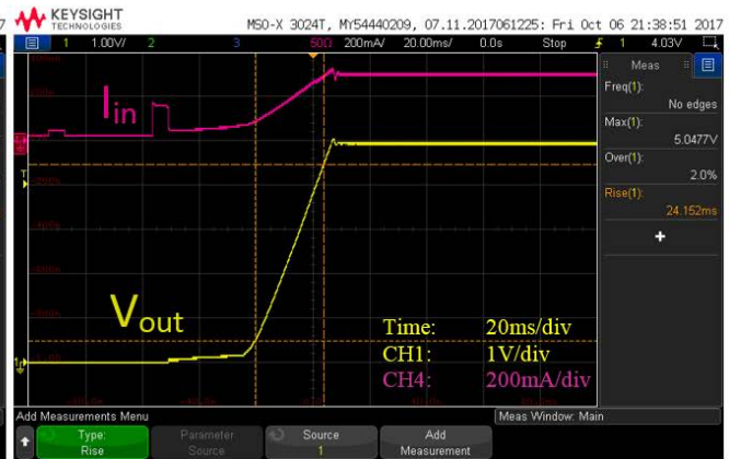
Figure 8.1. Si3404 Isolated Flyback EVB Output Voltage Soft-Start at Low Load (Left) and Heavy Load (Right) Conditions
