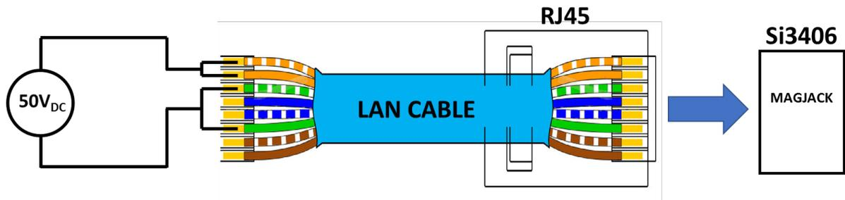
Figure 2.2. Midspan Connection using Laboratory Power Supply
