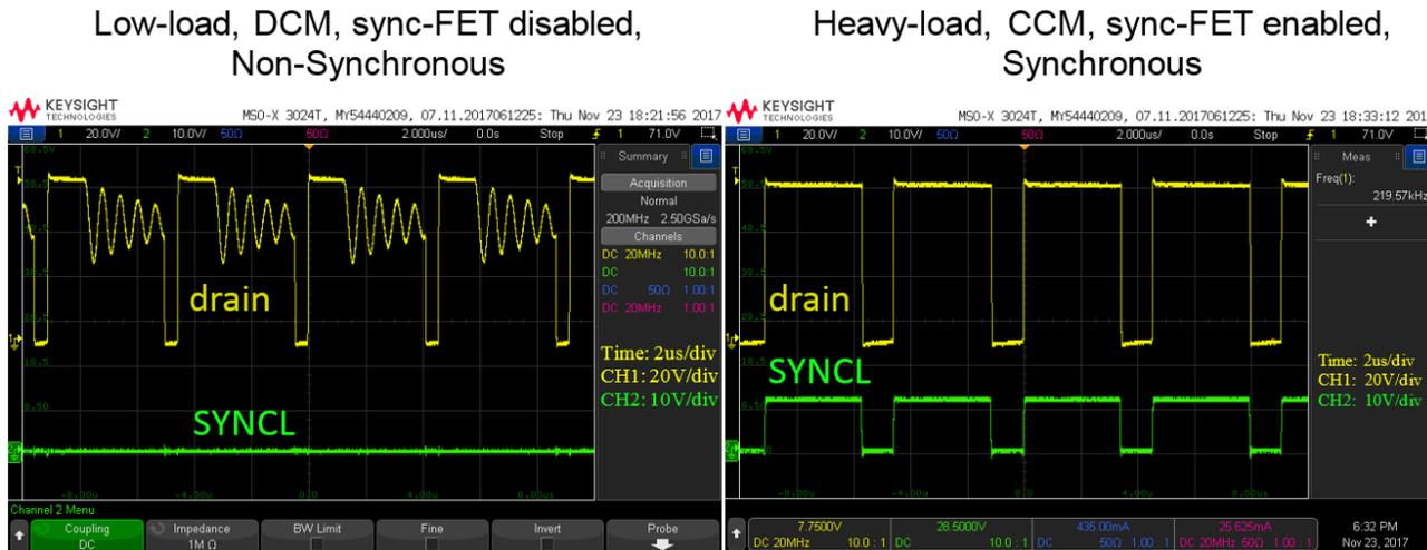
**Figure 13.1. DC-DC Switch Drain and SYNCL Voltage Waveforms at Discontinuous Current Mode (DCM) (Left) and in Continuous Current Mode (CCM) (Right)**
