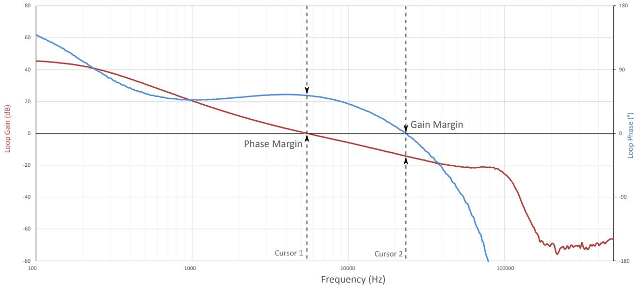
Figure 5.1. Si34061-ISO-FB EVB Measured Loop-Gain and Phase Shift
