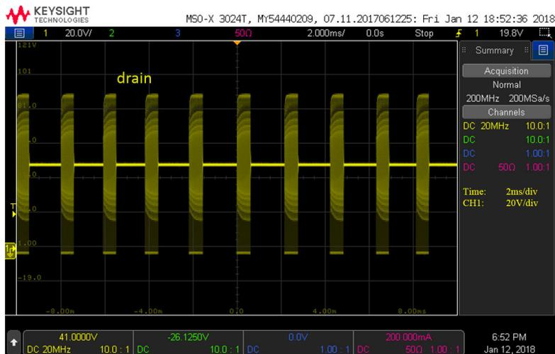
Figure 10.1. Si34061 Pulse Skipping at No-load Condition: SWO Waveform
