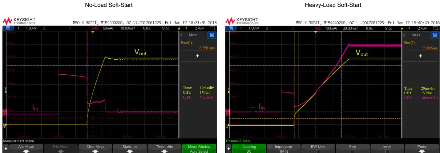
**Figure 8.1. Si34061 Isolated Flyback C4 EVB Input Current and Output Voltage Soft-Start at Low Load (Left) and Heavy Load (Right) Conditions**
