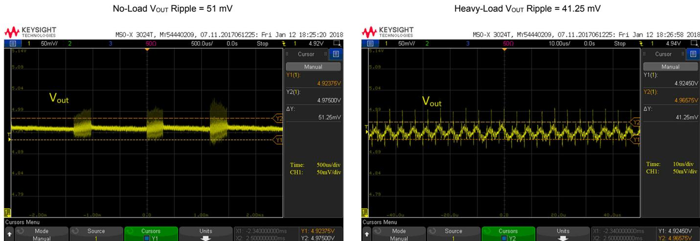
Figure 7.1. Si34061-Isolated Flyback C4 EVB Output Voltage Ripple No Load (Left) and Heavy Load (Right) Conditions
