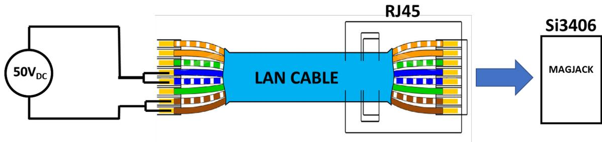
Figure 2.1. Endspan Connection using Laboratory Power Supply
