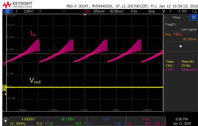
Figure 9.1. Si34061-Isolated Flyback C4 EVB Output Voltage and Input Current when Output is Shorted
