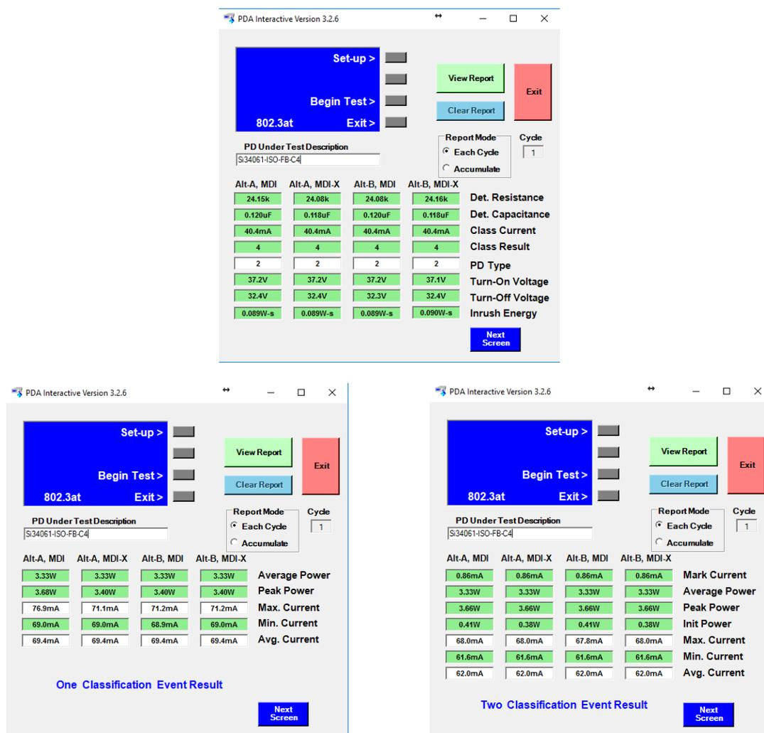
Figure 4.1. Si34061-Isolated Flyback C4 PD SIFOS PoE Compatibility Test Results
