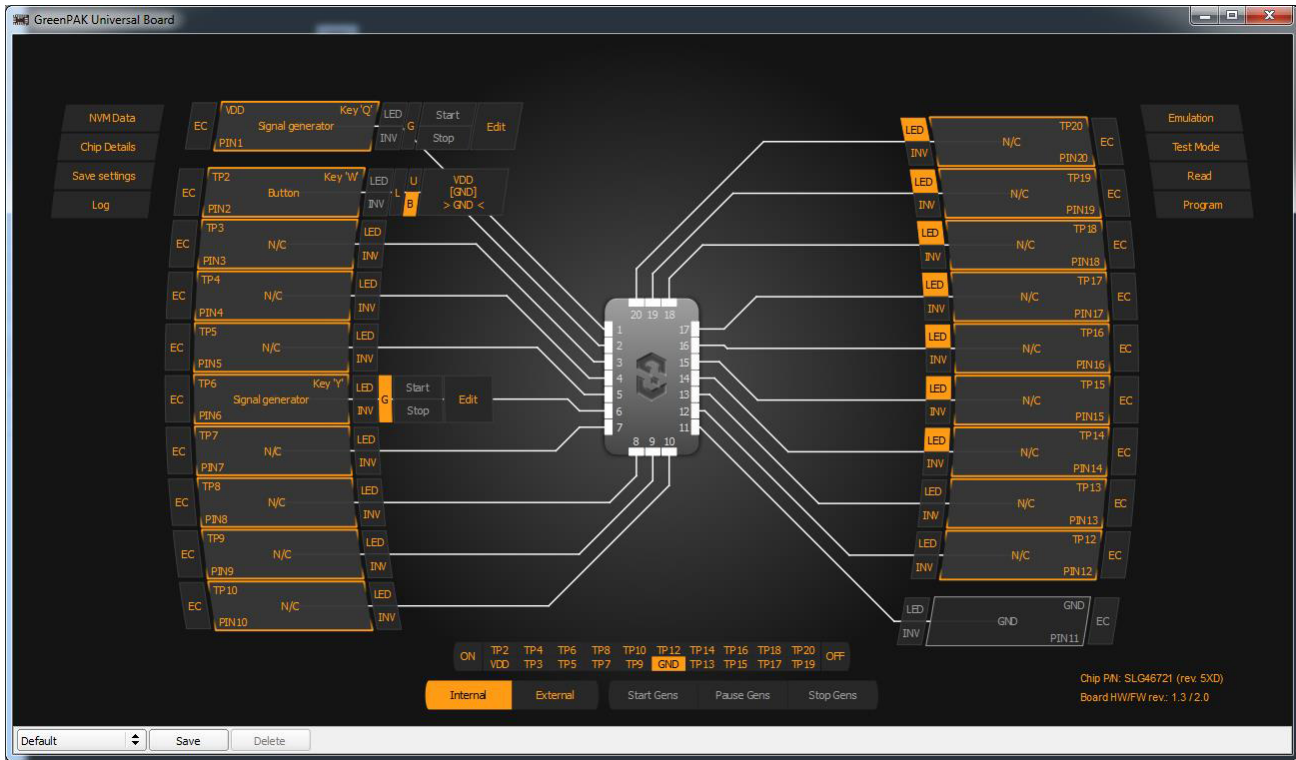
Figure 25. Emulation Window, with Buffered LED and Signal Generator
