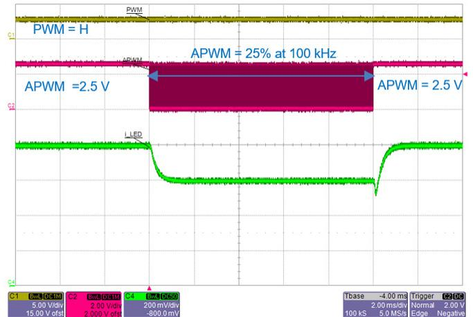
**Figure 28: PWM = H. Total LED current drops from  $400\text{ mA}$  ( $4 \times 100\text{ mA/ch}$ ) to  $300\text{ mA}$  when APWM of  $25\%$  duty cycle is applied. Note that LED current takes  $\sim 0.5\text{ ms}$  to settle after change in APWM.**
