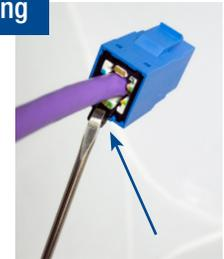
To remove, press down on the latch with a small screwdriver (or Belden release tool) and pull the cable out
