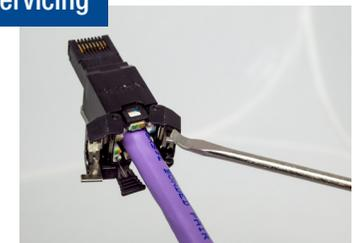
To remove, open the rear doors by squeezing the upper and lower pins. Lift on the latch with a small screwdriver (or Belden release tool) and pull the cable out
