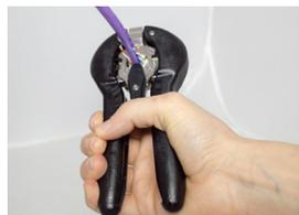
While holding the cable with one hand, compress the handles to complete your termination
