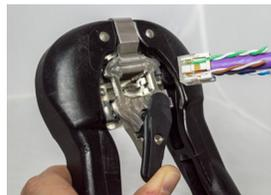
Insert the terminated core (cable manager and cap) into the tool until the middle latch returns to the center.
