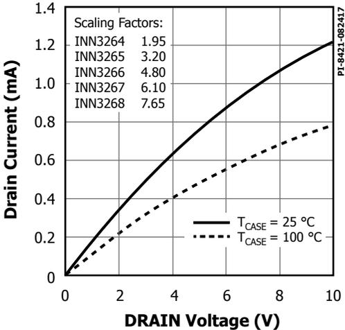
Figure 23. Output Characteristics.
