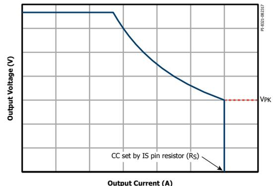
Figure 3. Typical Constant Power Characteristics.
