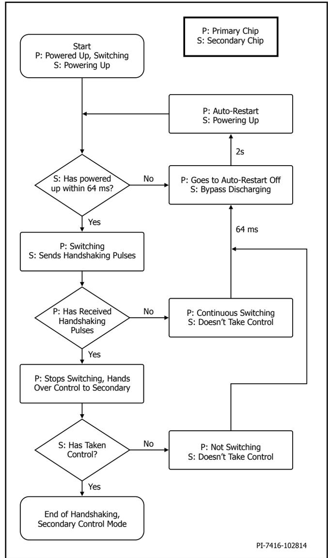
Figure 8. Primary-Secondary Handshake Flowchart.
