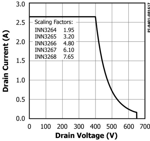
Figure 22. Maximum Allowable Drain Current vs. Drain Voltage.
