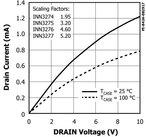
Figure 29. Output Characteristics.
