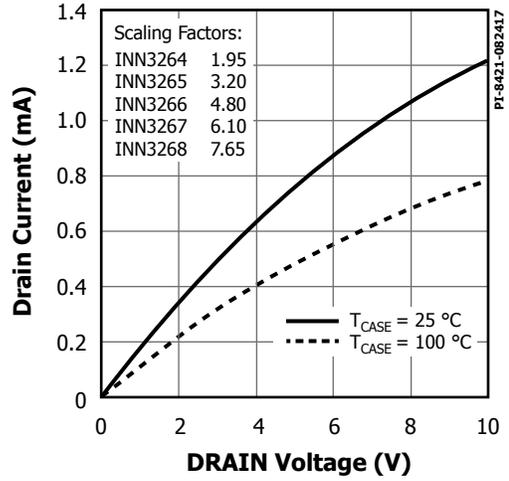
Figure 23. Output Characteristics.
