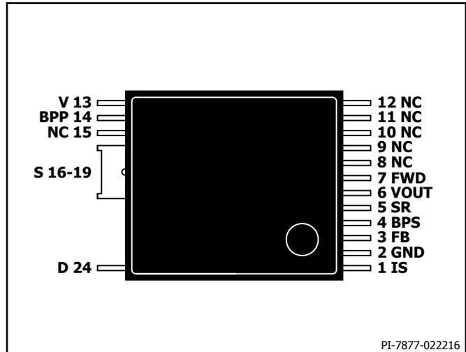
Figure 6. Pin Configuration.
