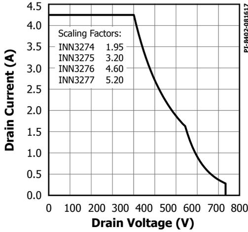
Figure 28. Maximum Allowable Drain Current vs. Drain Voltage.
