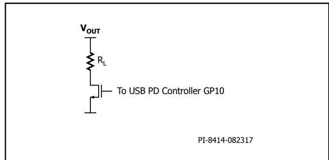
Figure 12. Active Pre-Load Circuit.
