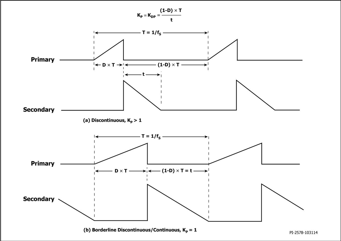
Figure 21. Discontinuous Conduction Mode Current Waveform,  $K_p > 1$ .
