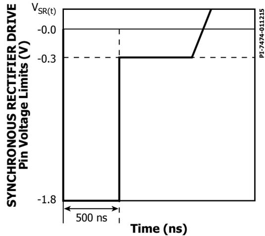
Figure 27. SYNCHRONOUS RECTIFIER DRIVE Pin Negative Voltage.
