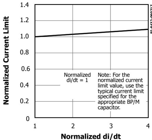
Figure 32. Standard Current Limit vs.  $di/dt$ .
