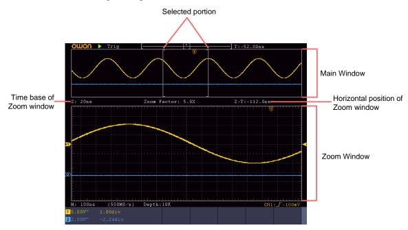
In normal mode, the **Horizontal Position** and **Horizontal Scale** rotary controls are used to adjust the horizontal position and time base of the Main window.
