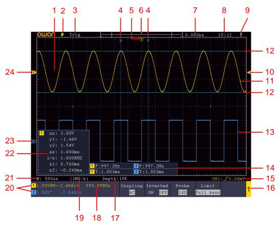
Figure 3-5 Illustrative Drawing of Display Interfaces
