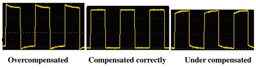
Figure 3-6 Displayed Waveforms of the Probe Compensation
