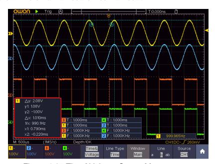
Figure 4-27 Time&Voltage Cursor Measurement
