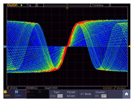
Figure 4-12 The color temperature function is on
