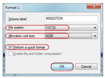
Figure 4-15: Formatting the USB disk setting
