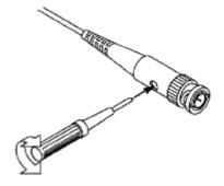
Figure 3-7 Adjust Probe
