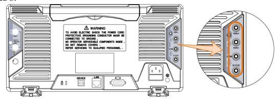
Figure 6-1 Multimeter Input Terminals
