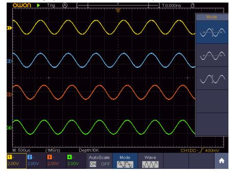
Figure 4-29 Autoscale Horizontal-Vertical multi-period waveforms
