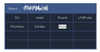
(4) Turn the **M** rotary control to select the desired waveform (or touch if the LCD is touchscreen). E.g. select **Noise**. Select **Select** to output the noise waveform.
