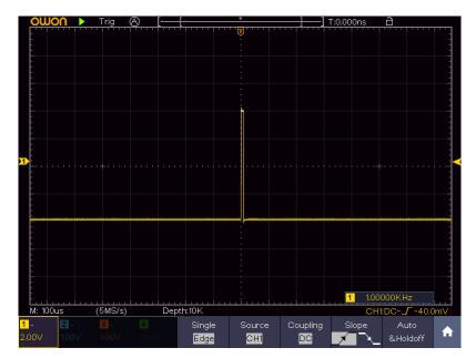
Figure 9-3 Capturing a Single Signal
