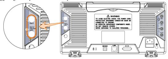
Figure 5-1 Generator Output Ports (Dual-channel)
