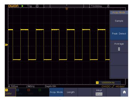
Figure 9-4 Signal with Noises
