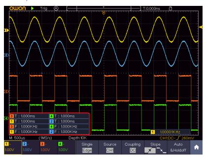
Figure 4-24 Automatic measurement
