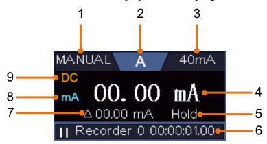
Figure 6-3 Multimeter Information Window
