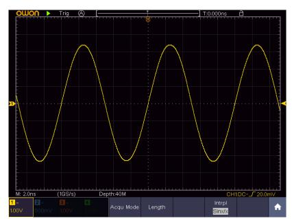
Figure 4-10 Sine(x)/x interpolation
