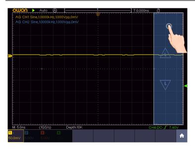
When the L icon appears, in the full screen, swipe up/down to control the trigger level of the source in the trigger menu.
