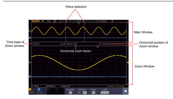
Figure 4-8 Waveform Horizontal Zooming Mode
