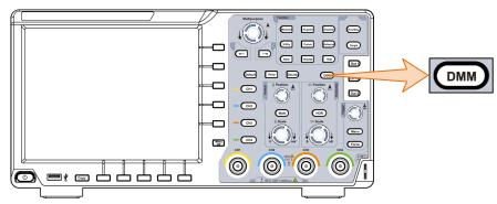
Figure 6-2 Multimeter Button
