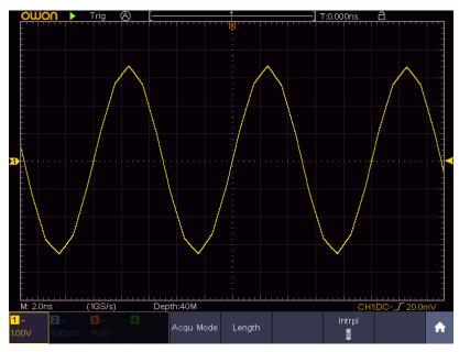
Figure 4-11 Linear interpolation
