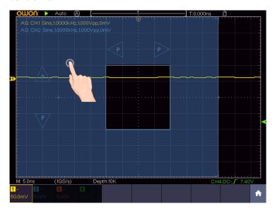
When the P icon appears, in the full screen, swipe left/right to control the horizontal position, swipe up/down to control the vertical position of the selected channel.
