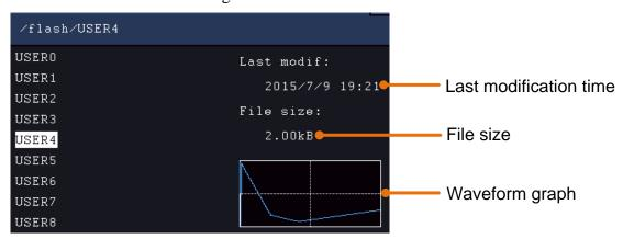
If a USB device is connected, and you want to save the waveform to it, select **Memory** in the right menu as **USB**. The instrument lists a directory of the folders and files on the USB memory device. Select a folder or file using the **M** rotary control to scroll up and down the list. To enter the current folder, select **Change Dir** in the right menu, select it again to return to the upper directory.
