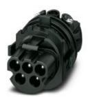
Circular connectors (cable-side), Contact insert, housing material: PPE, color: black, number of positions: 5, min. conductor cross section: 1.5 mm², max. conductor cross section: 6 mm², nom. voltage: 690 V AC, rated current: 35 A, Connection method: Screw connection, Type of contact: Pin
