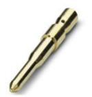
Crimp contact, leading (PE), turned, contact diameter: 1.5 mm, crimp range: 0.5 mm<sup>2</sup> ... 1 mm<sup>2</sup>
