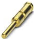
Crimp contact, turned, contact diameter: 2 mm, crimp range: 0.25 mm<sup>2</sup> ... 1 mm<sup>2</sup>
