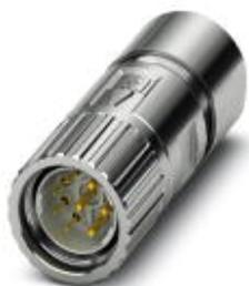
Cable connector, straight long, shielded: yes, Screw locking, M23, No. of pos.: 4+3+PE, type of contact: Pin, Crimp, cable diameter range: 7.5 mm ... 17 mm
