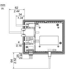
**NOTE:** All the above values are designed with cable bending in mind. The dimensions given here are representative values depending on the type of connection cable in use. Therefore, these values are intended for reference only.
