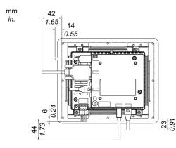
**NOTE:** All the above values are designed with cable bending in mind. The dimensions given here are representative values depending on the type of connection cable in use. Therefore, these values are intended for reference only.
