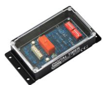
Timer with adjustable times between 1 second and 2047 seconds or 1 minute and 2047 minutes. The timer switches on after pressing the key and switches off again when the adjusted time has elapsed. The time lapse may be stopped at any time by using a second key. External push-buttons may be connected (not included). The timer can also be started by external control pulses (3 - 24 V / DC) or automatically after switching on with the connection of an Elko (22  $\mu\text{F}$  50 V).
