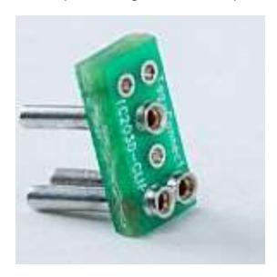
The Tag-Connect Clip Board (TC2030-CLIP-3PACK) attaches to the alignment pins of a Tag-Connect No Legs cable such as TC2030-MCP-NL. The Clip Board can be pressed onto the alignment pins from underneath the circuit board, providing a temporary connection for debugging purposes. Then you have the best of both worlds: a small PCB footprint and a reliable debugging connection.
