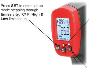
Press **MAX/MIN** to display these measurements on the LCD. When thermometer enters user set up mode use ▼ to select a further option.
