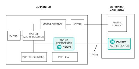
Figure 3. 3D printer cartridge authentication
