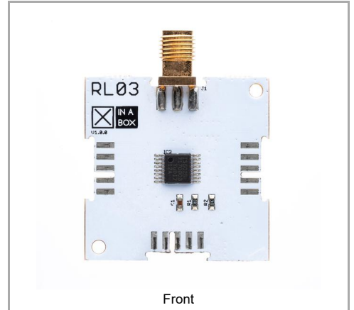
RL03 - LoRa Radio (915 MHz) (RFM96W/RFM95, SC18IS602B)
