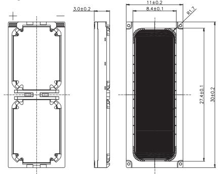
Dimensions : Millimetres Tolerance: ±0.2mm
