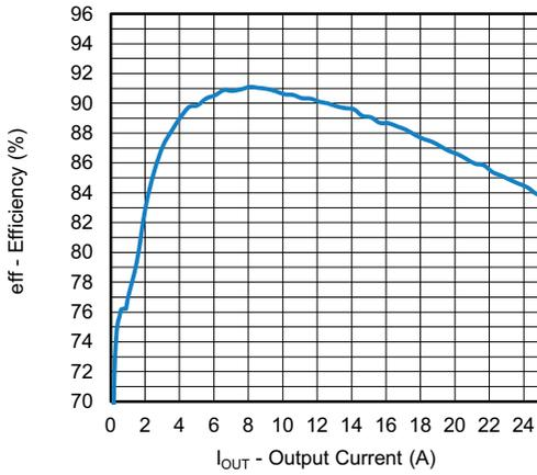
Fig. 11 - Efficiency vs. Output Current
