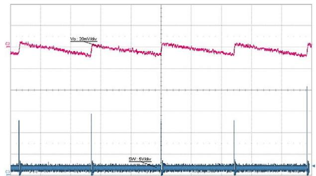
**Fig. 28 - Output Ripple, 0.01 A,  $t = 1 \mu$ s/div. DCM Mode**
