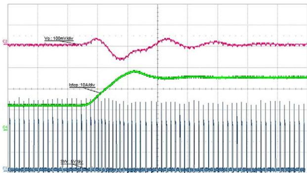
Fig. 19 - Load Step, 12 A to 25 A,  $1 \text{ A}/\mu\text{s}$ ,  $t = 10 \mu\text{s/div}$ .
