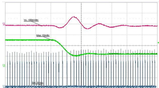
Fig. 22 - Load Release, 25 A to 12 A,  $1 \text{ A}/\mu\text{s}$ ,  $t = 10 \mu\text{s/div}$ .
