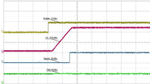
Fig. 17 - Startup With EN,  $t = 5 \text{ ms/div}$ .
