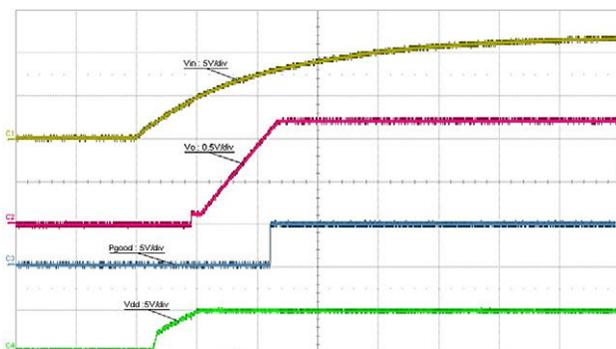
Fig. 13 - Startup With  $V_{IN}$ ,  $t = 5\text{ ms/div}$ .
