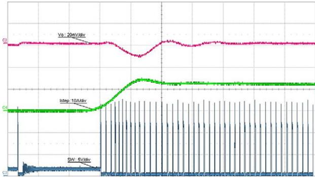
**Fig. 23 - Load Step, 0.1 A to 12 A, 1 A/ $\mu$ s,  $t = 10 \mu$ s/div. Skip Mode Enabled**
