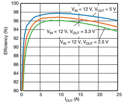
**Fig. 2 - Efficiency vs. Output Current**
