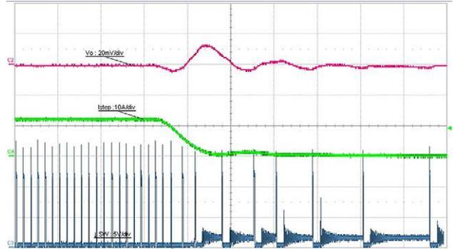
**Fig. 26 - Load Release, 12 A to 0.1 A, 1 A/ $\mu$ s,  $t = 10 \mu$ s/div. Skip Mode Enabled**
