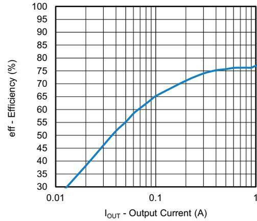
Fig. 14 - Efficiency vs. Output Current - Light Load
