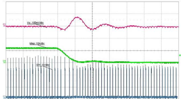
**Fig. 27 - Load Release, 12 A to 0.1 A, 1 A/ $\mu$ s,  $t = 10 \mu$ s/div. Forced Continuous Conduction Mode**
