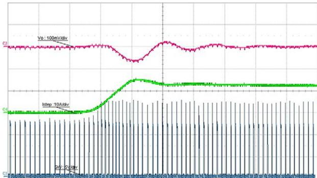
**Fig. 24 - Load Step, 0.1 A to 12 A, 1 A/ $\mu$ s,  $t = 10 \mu$ s/div. Forced Continuous Conduction Mode**
