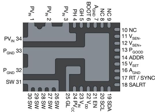
**Fig. 4 - Pin Configuration - Bottom View**
