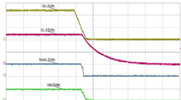
Fig. 16 - Shut Down With  $V_{IN}$ ,  $t = 100\text{ ms/div}$ .
