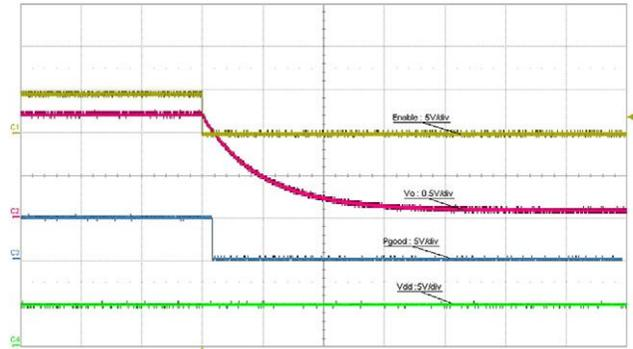
Fig. 20 - Shut Down With EN,  $t = 100 \text{ ms/div}$ .
