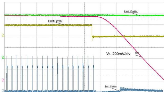
Fig. 18 - Overcurrent Protection Behavior,  $t = 5 \mu\text{s/div}$ .
