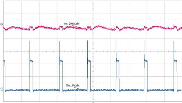
**Fig. 29 - Output Ripple, 12 A, t = 1  $\mu$ s/div.**
