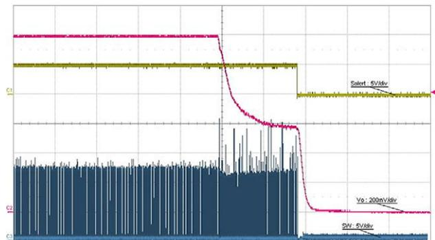
Fig. 21 - Output Undervoltage Protection Behavior,  $t = 100 \mu\text{s/div}$ .
