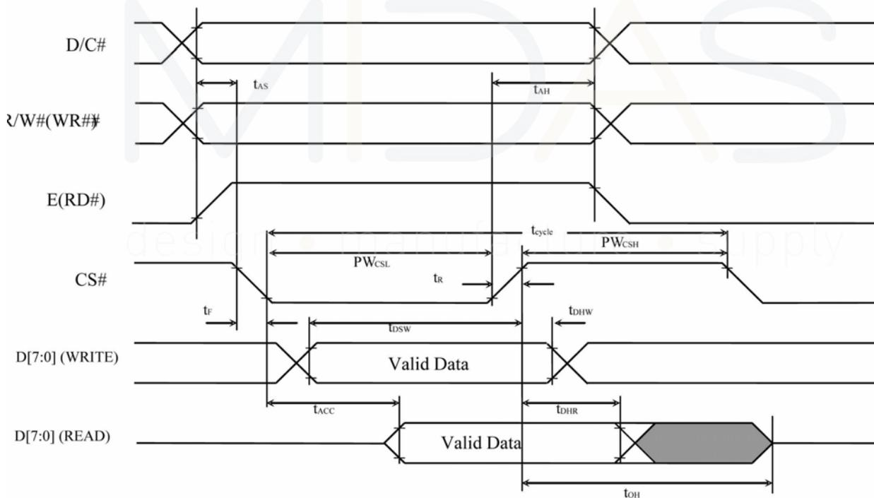
**Table 13-3 : 8080-Series MCU Parallel Interface Timing Characteristics**
