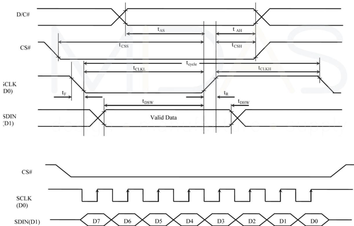
**Table 13-5: Serial Interface Timing Characteristics (3-wire SPI)**
