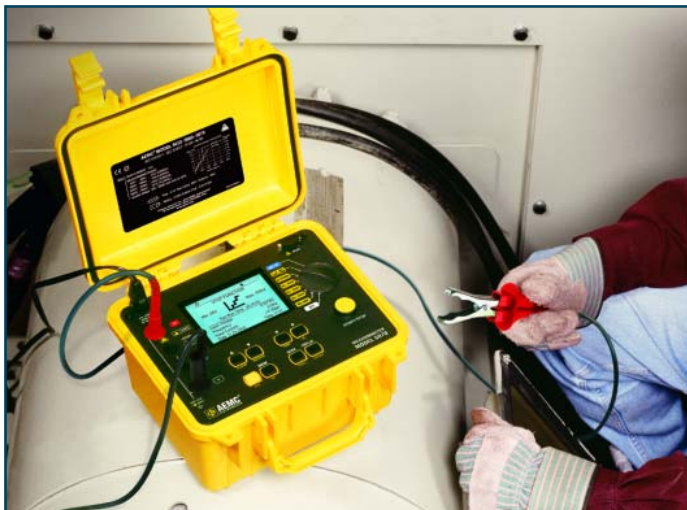
Model 5070 performing insulation test on a generator.
