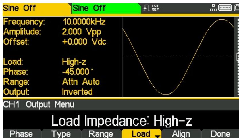
The default load impedance is 50 Ohms, but that this could be changed to any impedance between 50 and 10,000 Ohms. Levels are calculated based upon this impedance.
