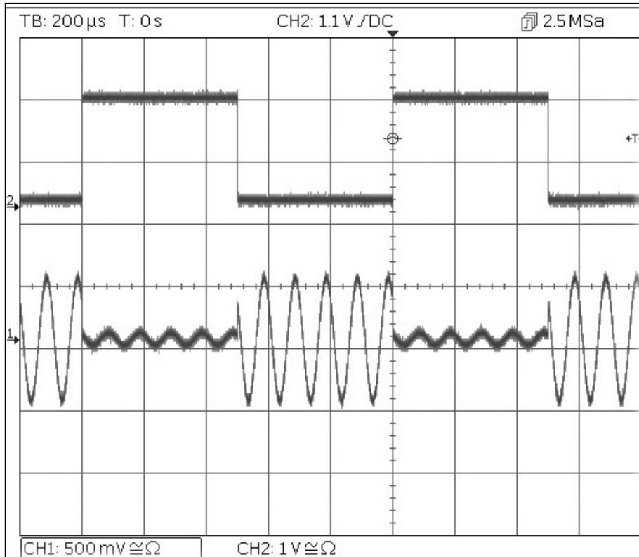
Note that the second trace is the output from the main Output 2 socket when Channel 2 is synchronised which follows the modulating waveform signal.
