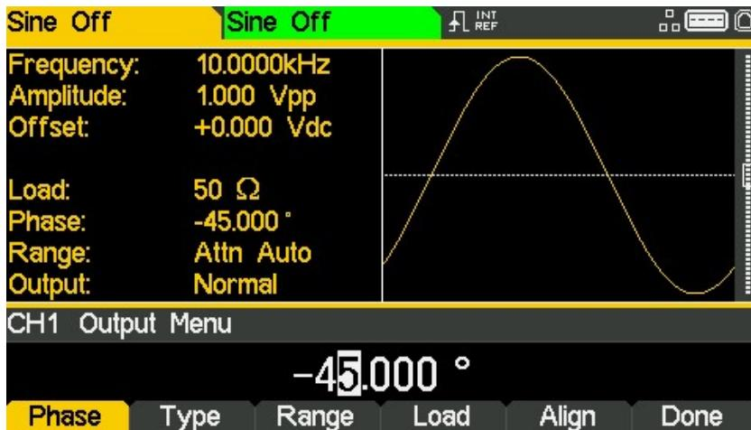
The set phase angle is the point in the waveform period which is coincident with the Sync or trigger edge, i.e. it is the point in the period at which the waveform starts. Hence a negative phase setting advances, and a positive phase setting delays the waveform relative to the Sync or trigger; the waveform in the graph box changes to show this.
