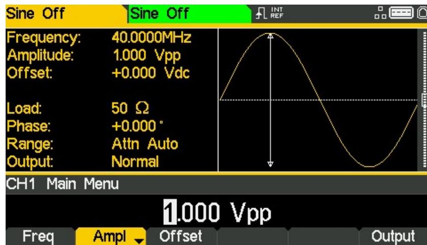
Successive presses of the Ampl soft-key changes the Ampl and Offset key labels to HiLvl (high level) and LoLvl (low level) and vice versa.
