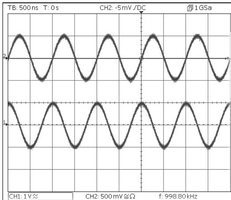
Note that, when channel 1 is set to 1MHz, channel 2 is also set to 1MHz.
