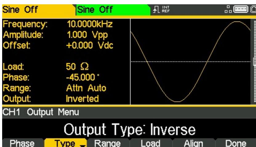
Successive presses of the type key alternates between normal and inverted.
