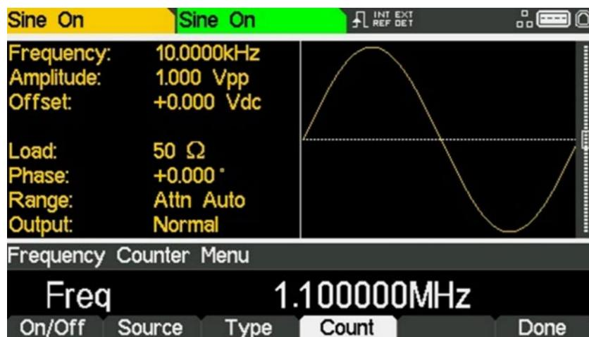
The Edit Box shows the current measurement. With no input signal at the selected input, the counter displays 'No signal' until an adequate input signal is applied. When an adequate input signal is applied, the counter constantly measures and displays the reading in the Edit Box.
