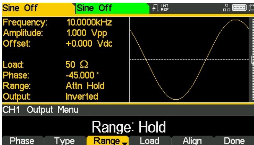
Auto mode auto-ranges in 6dB attenuator steps (i.e. 'range' maximums of 10Vpp, 5Vpp, 2.5Vpp, etc., into 50Ω), with the amplitude range limited to 6dB to maintain waveform quality.
