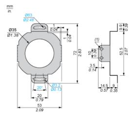
(1) 4 holes Ø 3.2. M3 x 6 screw fixings.
