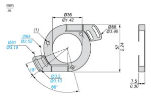
(1) 3 holes Ø 4.1 at 120° on 48 PCD. TC M3 x 6 screw fixings
