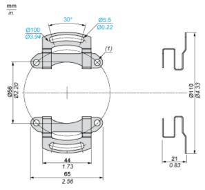
(1) 4 holes  $\varnothing$  5.2 at 90° on 78 PCD. TH M5 x 6 screw fixings
