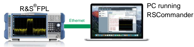
Fig. 3-3: LAN instruments connected to PC
