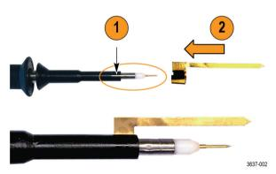
Connecting the Y-lead adapter and micro-SMD clip. The browser kit includes a Y-lead adapter and a micro-SMD clip that connect as shown below. The Y-lead adapter can also connect to square pins
