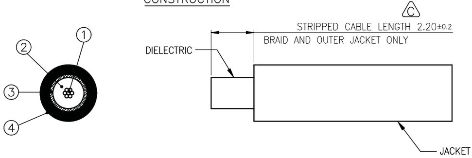
NOTE: JACKET STRIP OD DEFORMED MUST BE THAN LESS  $\phi 3.30\text{mm}$  AFTER CUT OFF.
