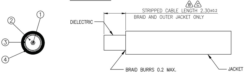
NOTE: JACKET STRIP OD DEFORMED MUST BE THAN LESS  $\phi 2.75\text{mm}$  AFTER CUT OFF.
