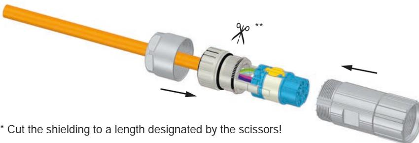
\*\* Cut the shielding to a length designated by the scissors!
