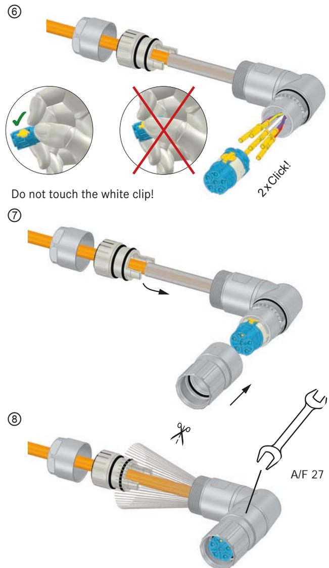
Cut the shielding to a length designated by the scissors and position the edge of the shielding between the two O-rings (refer to red arrow in step ⑧).
