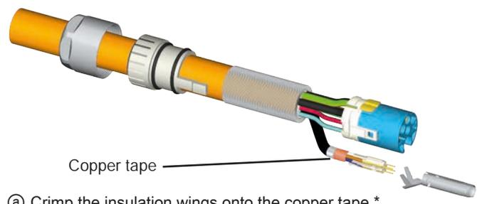
ⓐ Crimp the insulation wings onto the copper tape.\*
