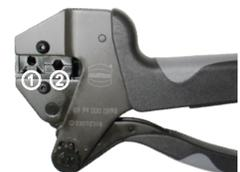
ⓑ Crimp the shielding sleeve, overlapping the insulation crimp.\*\*
