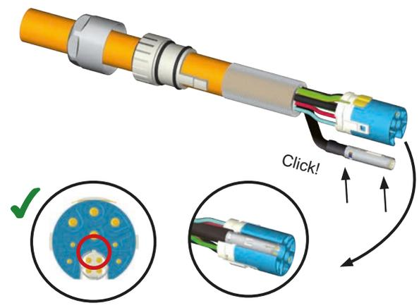
⑬ Push the latching hooks of the cable gland body through the shielding and let them snap into place on the insert (⇒ white ring slot).
