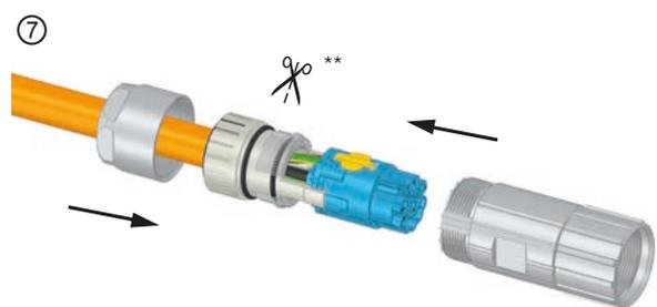
\*\* Cut the shielding to a length designated by the scissors.
