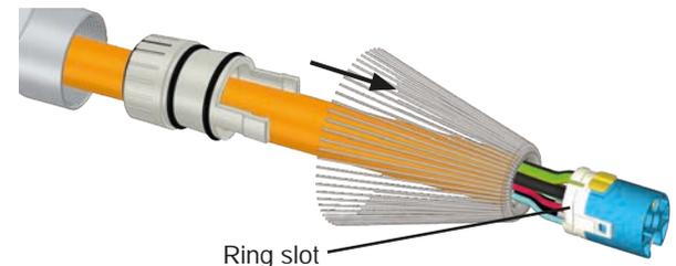
⑭ Strip the shielding between the first and the second O-ring!
