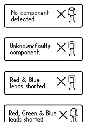
It is possible that the *DCA Pro* may detect one or more diode junctions or other component type within an unknown or faulty part. This is because many semiconductors comprise of PN (diode) junctions. Please refer to the section on diodes and diode networks for more information.
