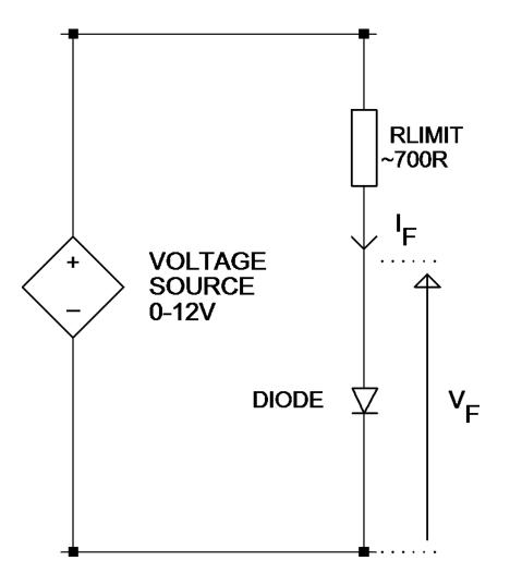
This test circuit is used for testing both the forward and reverse characteristics of diodes. Reverse characteristics are particularly useful for the testing of Zener diodes.
