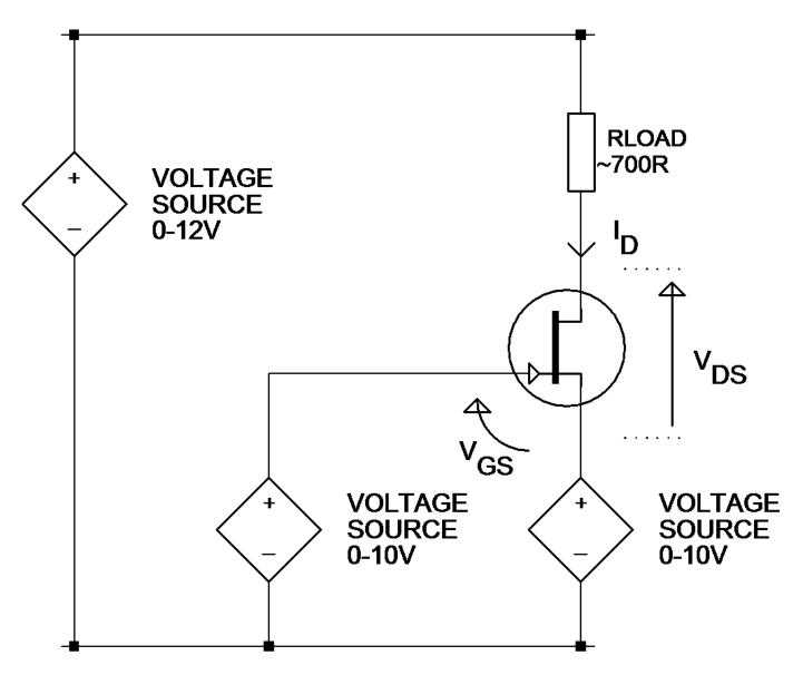
It's important to note that the gate-source voltage can be driven negative by making the source voltage drive higher than the gate voltage drive. When this is done however, there is less voltage available to be across the drain-source nodes and the load resistor.
