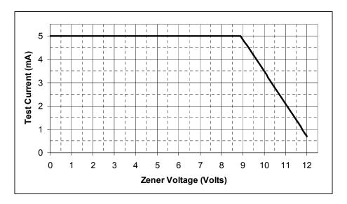
\*The *DCA Pro* may not be able to identify Zener diodes with a Zener voltage of more than 11V. It will however still identify the diode junction in its forward biased mode.
