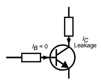
Older Germanium types however can suffer from significant collector leakage
