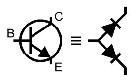
junction represents the base terminal. This is normal for situations where the current gain is so low that it is immeasurable at the test currents used by the *DCA Pro*.
