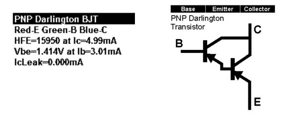
Note that the component schematic is displayed in colour to illustrate which colour test lead is connected to each component lead.
