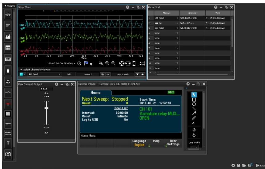
Figure 2. BenchVue's data visualization tools (an example of strip chart, data grid, D/A current output and add screen image tool)
